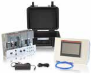
AC500 basic training case CPU, I/Os, HMI
