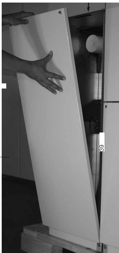
2. Pull out and lift the cover off
