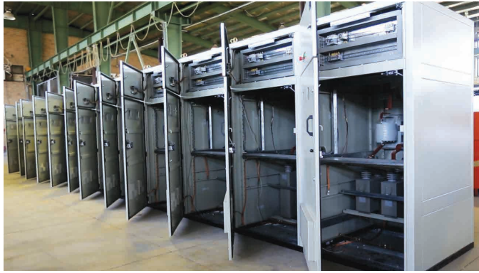
MV Capacitor Bank
