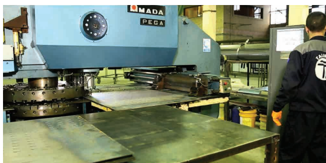
CNC Hydraulic Punching Machine
